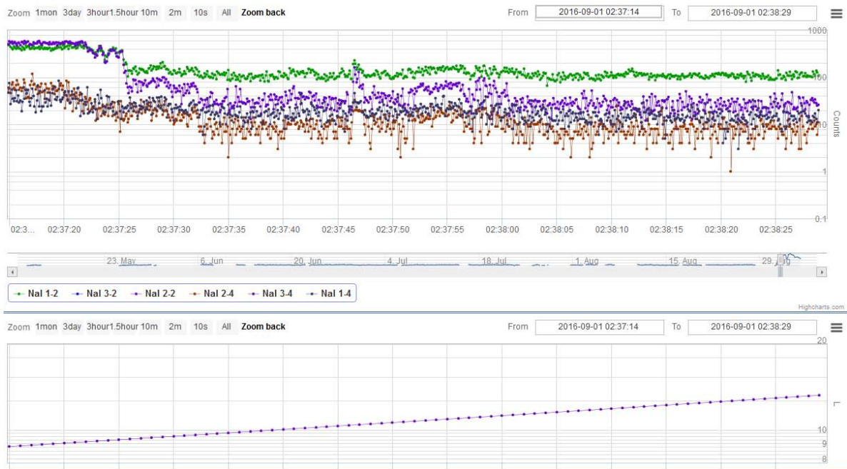
Fig. 4. The time profiles of counting rates in BDRG Lomonosov channels, BDRG-1 20 – 35 keV (green line), BDRG-3 20-35 keV (lilac line), BDRG-1 60 – 100 keV (blue line), BDRG-3 60 – 100 keV (brown line). Time scale means universal time UT. The middle panel: the time profile of L values at the same times as on the top panel.
